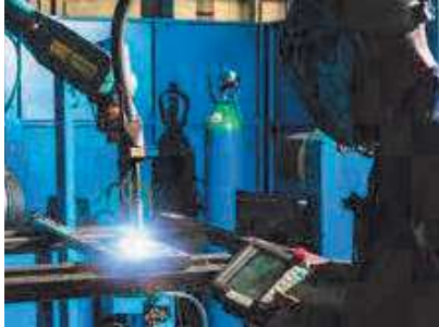
Robotic MAG welding
