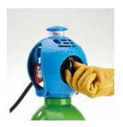
4 Set the outlet pressure or flow rate
